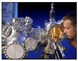
The microscope must be kept under high vacuum and exceptionally cold.
